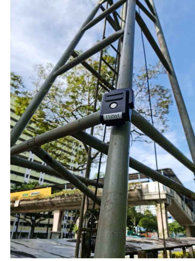
Geofencing and tracking digging equipment
